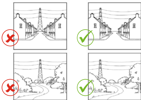
Offsetting the views of pylons will help make them less prominent ( 'A Sense of Place: Design Guidelines for development near high voltage overhead lines' – National Grid, page 36 )
